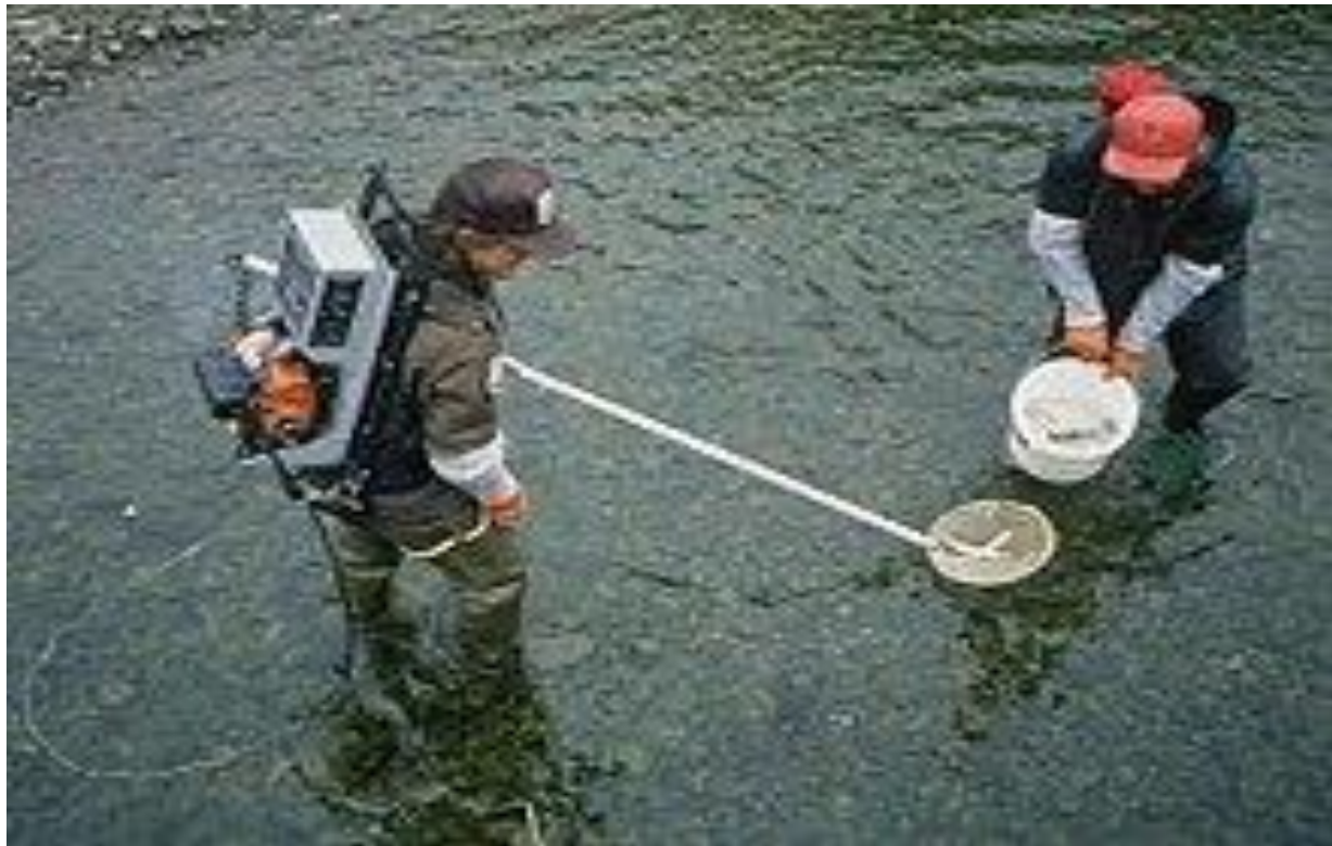
Figure 4: Electro fishing survey methods use a mild electric shock to temporarily stun fish for capture, identification and counting. The fish are then returned to the water unharmed.
